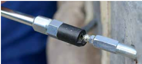
Slide DESOI Snappy onto the round head nipple, locking bar at the bottom
